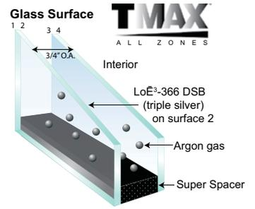
Low E insulated glass packages are a great option to help you reduce your heating and cooling costs. In warm weather, Low E glass reduces solar heat gain, minimizes interior glare and lowers inside glass temperature, saving energy. In cool weather, Low E glass provides outstanding thermal performance with warmer inside glass surfaces to help save energy.
